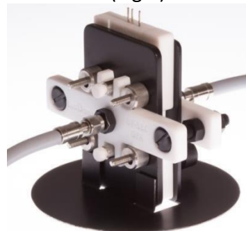
Figure 3: Spectroelectrochemical cell with optical fibres.
