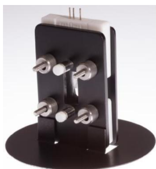
Figure 1: Thin-layer spectro-electrochemical cell (left). Zoom on the Electrode configuration, the so-called "spacer" (right).
