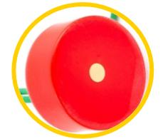
*Standard 5 mm Au disc sample measured with tap water droplet for comparison*
