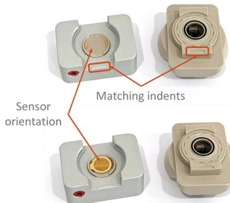
**2** With the cell open, place the sensor minding the orientation drawn in the sensor bed. Identify and align the matching indents in base and lid of the cell before closing the cell.
