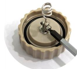
**4** Fix your electrode in the steel rods at the sides of the lid, or use the one placed in the inside face of the window lid.
