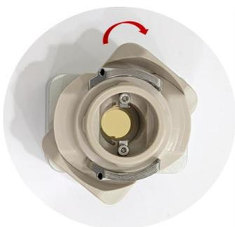
**3** To close the cell, first, push lightly the lid into the base (vertically) and then, rotate a quarter of a turn.
