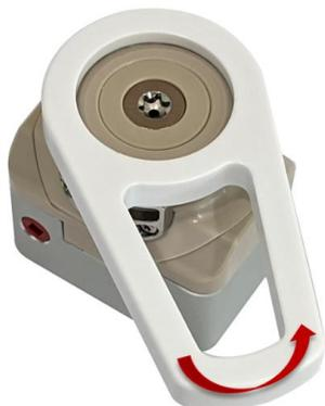
**1** Use the tool provided for opening the window lid before opening the cell.
