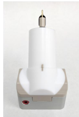
4 Insert electrode holder and place RE and CE
