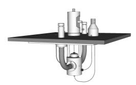
Fig. 1 : cryo-mixing chamber (below the plate)
