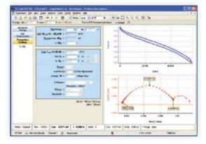
In case of fuel cell testing, the monitored current can be used to control gas flow meters thanks to the external device configuration window.
