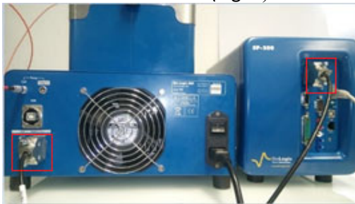
Figure 3: Connection of the potentiostat board to an ITS using the DB9-DB9 cable.
