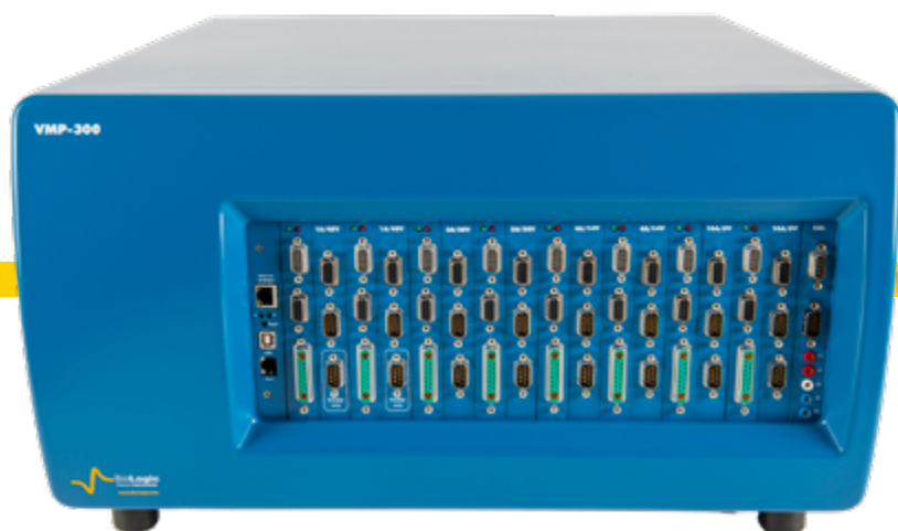
VMP-300 16 channels, \pm 150 A down to 100 fA
