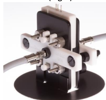
Figure 3: Spectroelectrochemical cell with optical fibres.
