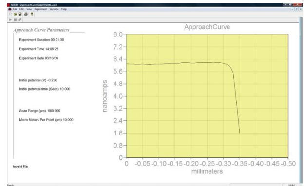
Figure 4 : Approach curve to the screen printed surface.
