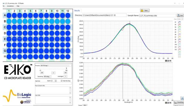
**Fig. 3. Raw CD spectra of CSA.** The CD spectra of 200  $\mu$ l H<sub>2</sub>O & (+) CSA (Sigma) at 3 mg/ml in wells #A1-H12 of a solid fused silica 96 well plate with black sidewalls (Hellma) from 240 - 340 nm were taken. Raw data was collected with no effort to minimize the noise or evaporation at a room temperature of 25°C. Representative data from cells B1-B12 are shown.
