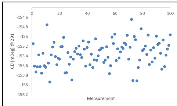
**Fig. 1. Consecutive measurements in in wells A10 & F2 of (-) CSA as a function of measurement.** Successive measurements of 200  $\mu$ l of (-) CSA (Sigma) at 1 mg/ml in wells #A10 & #F2 of a solid fused silica 96 well plate (Hellma) taken at 291 nm. Data was collected with no effort to minimize evaporation (samples were not protected with an optically clear cover) or reduce the noise (data were collected with the shortest integration times possible) at a room temperature of 25°C.
