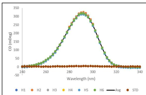
**Fig. 5. Raw CD spectra of CSA from the final row of wells of an unskilled technician.** The CD spectra of 200  $\mu$ l (+) CSA (Sigma) at 1 mg/ml in wells #H1-H6 of a solid silica bottom 96 well plate with black sidewalls (Porvair) from 240 - 340 nm were taken. Raw data were collected with no effort to minimize the noise or evaporation at a room temperature of 25°C. Wells H1-H6 are shown in addition to the mean and standard deviation of those six.
