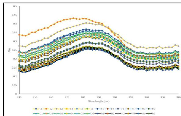
**Fig. 4. Absorbance determinations of CSA by an unskilled technician.** The Absorbance spectra of 200  $\mu$ l (+) CSA (Sigma) at 1 mg/ml in wells #A1-H12 of a solid silica bottom 96 well plate with black sidewalls (Porvair) from 240 - 340 nm were taken. Raw data were collected with no effort to minimize the noise or evaporation at a room temperature of 25°C. Representative data is shown in groupings of six and are color coded.
