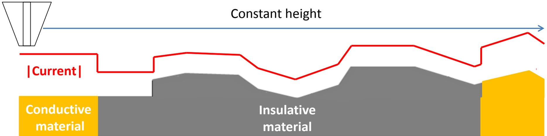
If both the conductivity and the topography of the substrate change, there is no way to discriminate their contribution to the current. The solution is to keep the electrode to sample distance constant. This can be done using Height Relief but it is using two techniques, two scans and a positional reference is needed.
