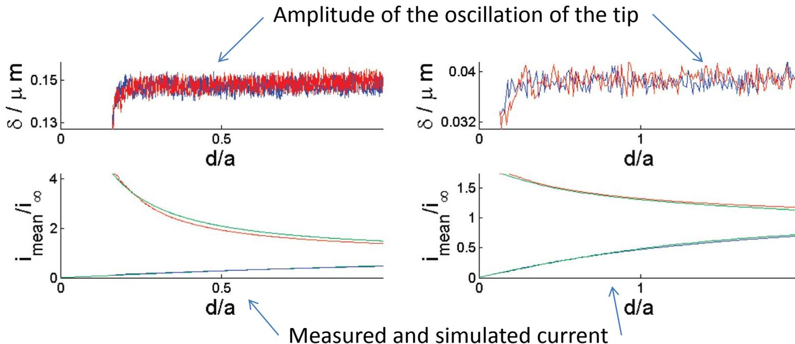
Feedback approach curves to conducting, gold (red), and nonconducting, glass (blue), substrates
