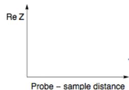
For low frequencies, or high conductivity electrolyte,  $Re Z$  increases when the tip approaches the surface.
