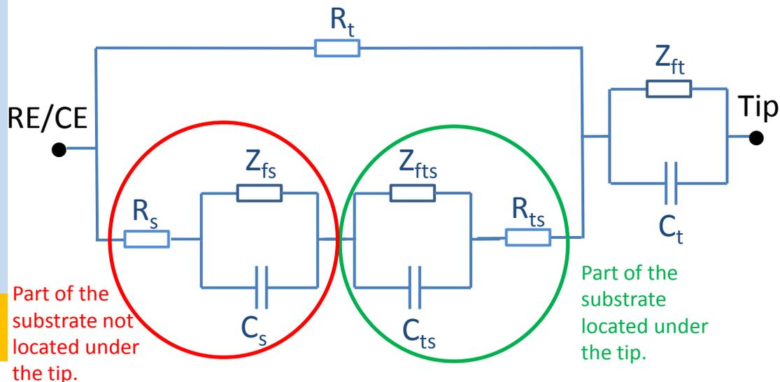
Now the current has two paths: either directly through the solution ( $I'$ ) or through the conductive substrate by crossing the substrate/electrolyte interface twice ( $I''$ ).
