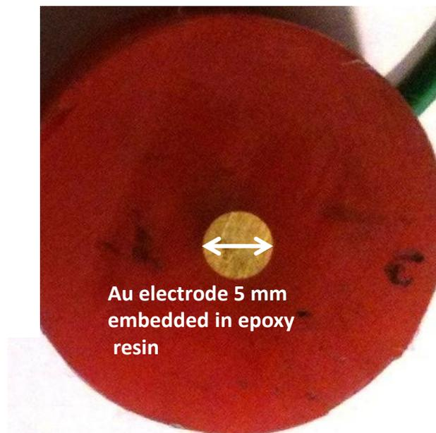
10 mM  $\text{Fe}^{\text{III}}/\text{Fe}^{\text{II}}$ , 100 mM KCl
