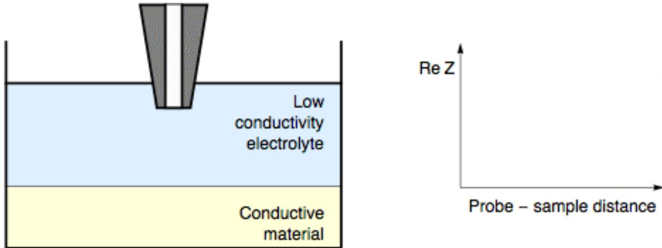
For high frequencies, or low conductivity electrolyte,  $\text{Re } Z$  decreases when the tip approaches the surface.
