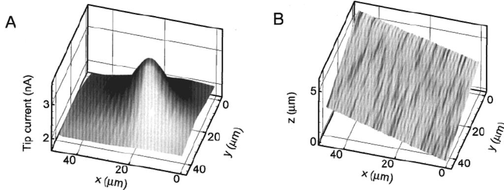
Feedback (A) and topographic (B) height images of a 10 μm diameter Pt disk substrate acquired under impedance feedback control
