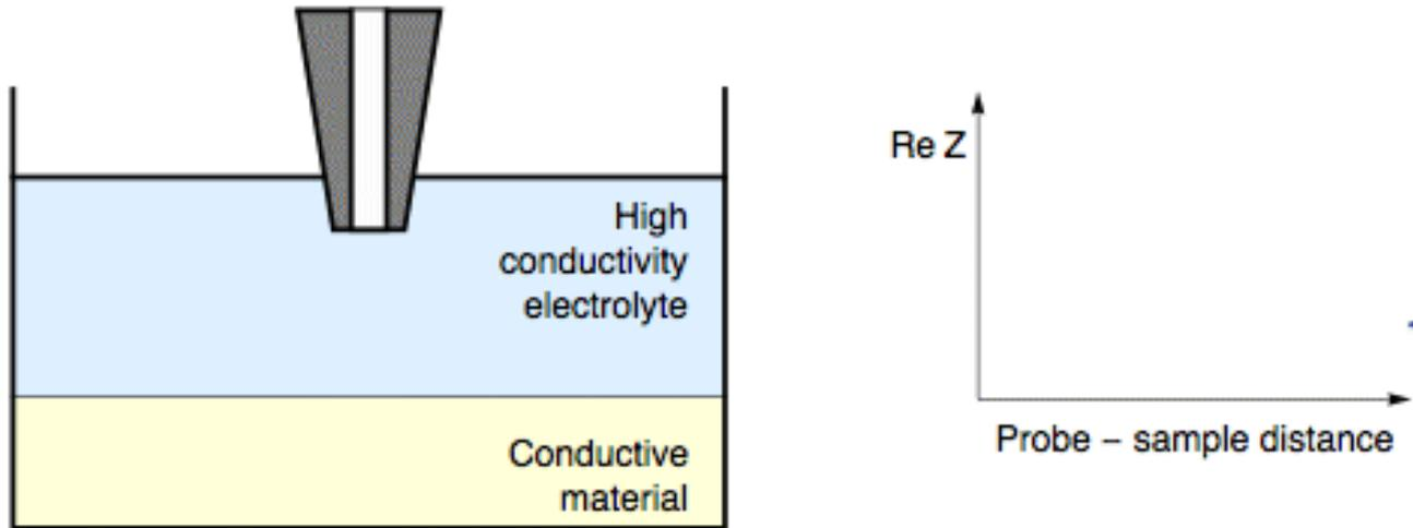
For low frequencies, or high conductivity electrolyte, Re Z increases when the tip approaches the surface.
