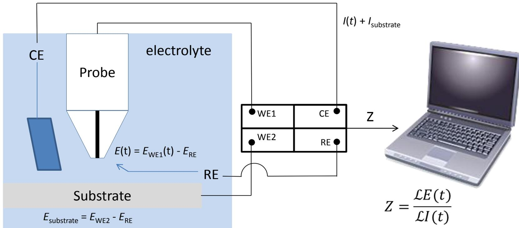
The electrochemical cell, comprised of the solution between the tip of the probe and the substrate, can be modelled using equivalent circuits.
