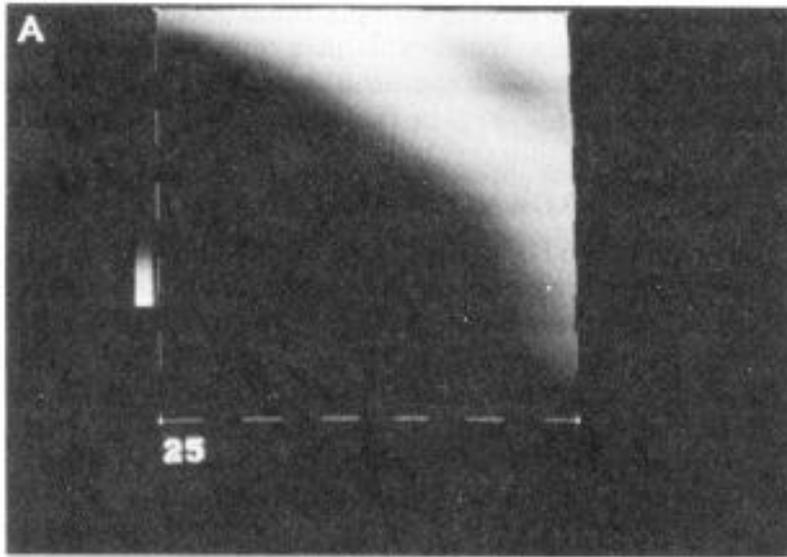
Image of the concentration profile of hydrogen peroxide near the surface of a glassy carbon-platinum composite.
