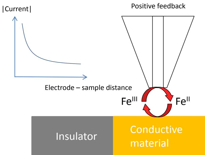
SECM requires the use of an electroactive species :  $FeCN_6^{3-}$ ,  $Ru(NH_3)_6^{3+}$ , which can interact with either the substrate for instance dissolved metal ions from corrosion or with the other species contained in the electrolyte *i.e.* corrosion inhibitors.
