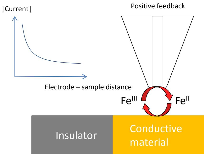
SECM requires the use of an electroactive species :  $\text{FeCN}_6^{3-}$ ,  $\text{Ru}(\text{NH}_3)_6^{3+}$ , which can interact with either the substrate for instance dissolved metal ions from corrosion or with the other species contained in the electrolyte *i.e.* corrosion inhibitors.
