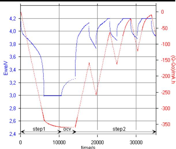
**Figure 1:  $E_{we}$  and  $(Q-Q_0)$  evolution versus time at the beginning of the experiment.**
