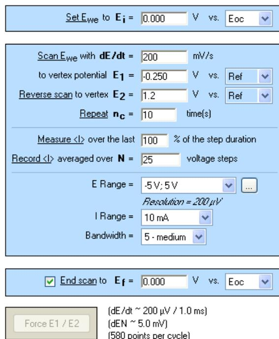
**Figure 1: Cyclic Voltammetry "Parameters Settings" window.**
