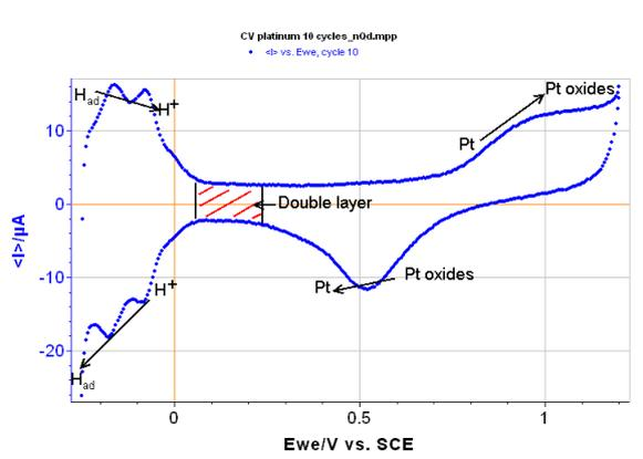
**Figure 3: 10<sup>th</sup> cycle isolated from the curve with oxo-reduction specificities for platinum.**
