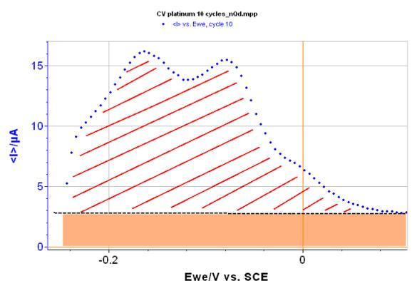
**Figure 4: Zoom of the curve presented in Figure 3 for low potentials in oxidation. The red area corresponds to the desorption of hydrogen. The orange area corresponds to the capacitive current due to the double layer capacitance.**
