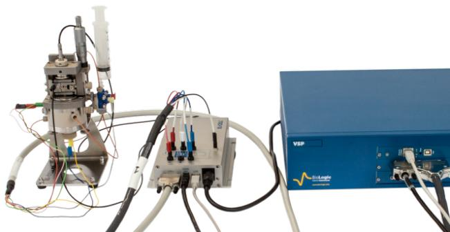
**Figure 3: Picture of the setup. Dilatometer (left), Data logger (center) & VSP (right).**
