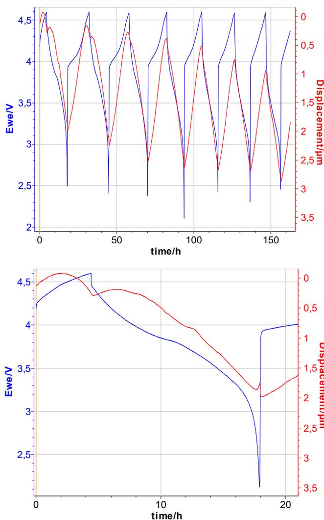
**Figure 7: Electrode potential and dilation evolution during constant current cycling of a  $\text{LiCoO}_2$  electrode. Bottom: focus on the phase transitions at the two vertex points and at the first discharge midpoint.**
