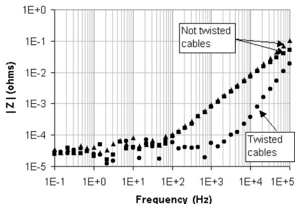
**Figure 6: Magnitude spectra of the magnetic coupling.**
