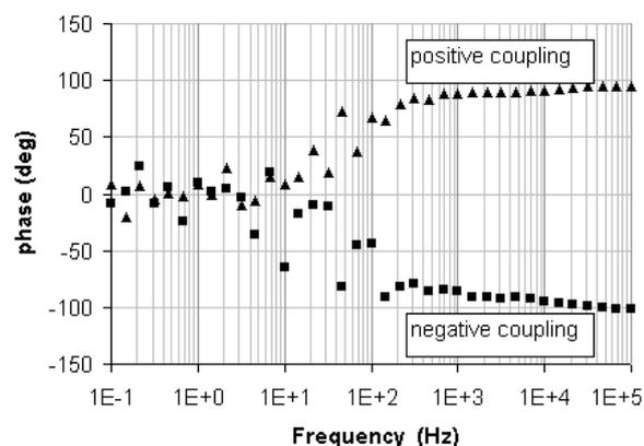
**Figure 7: Phase spectra of the magnetic coupling.**
