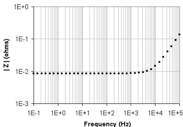
**Figure 4: Impedance data for a straight 10 cm wire.**
