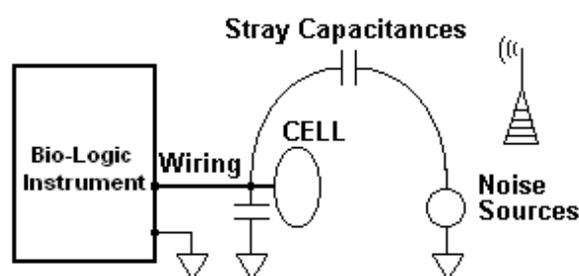
**Figure 1: Stray capacitances are related to wiring.**
