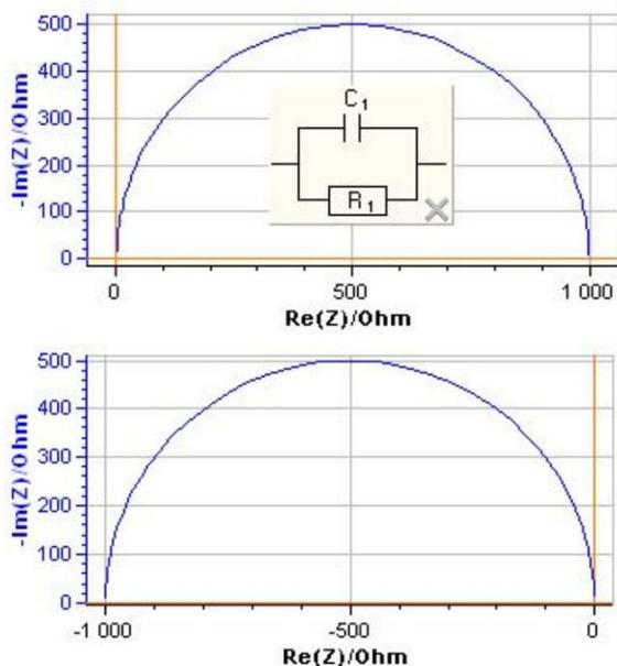
Figure 10: Nyquist diagrams for a RC parallel circuit.
