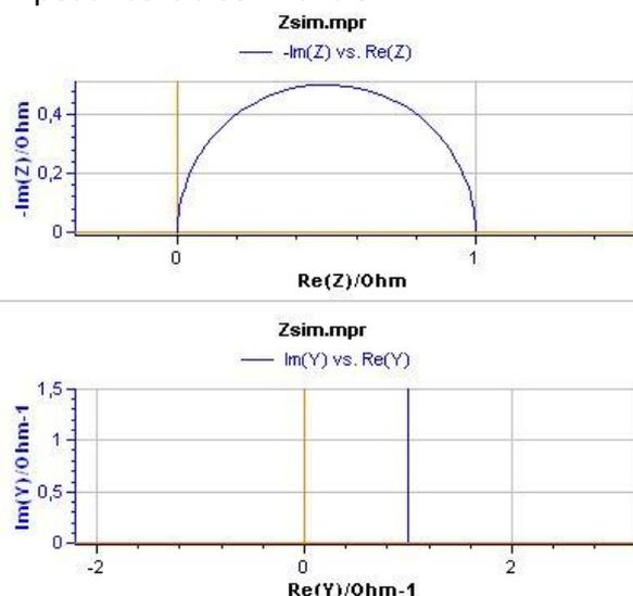
**Figure 6: Impedance and admittance diagrams of an RC parallel circuit.**
