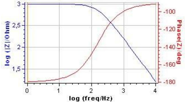
**Figure 8: Bode magnitude and phase plots for an RC parallel circuit.  $R = 10^3 \Omega$ ,  $C = 10^6 \text{ F}$ .**
