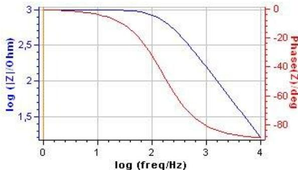
**Figure 7: Bode magnitude and phase plots for an RC parallel circuit.  $R = 10^3 \Omega$ ,  $C = 10^6 \text{ F}$ .**
