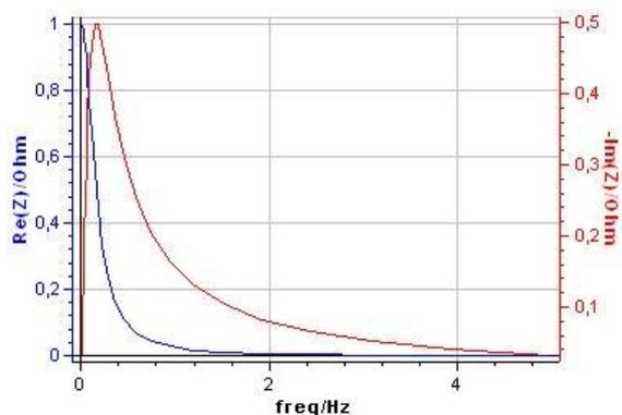
**Figure 2:** Plots of  $\text{Re } Z$  vs.  $f$  and  $\text{Im } Z$  vs.  $f$  for the RC parallel circuit.
