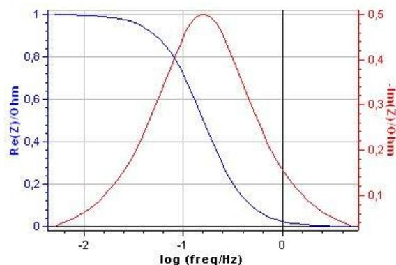
**Figure 3:** Plots of  $\text{Re } Z$  vs.  $\log f$  and  $\text{Im } Z$  vs.  $\log f$  for the RC parallel circuit.
