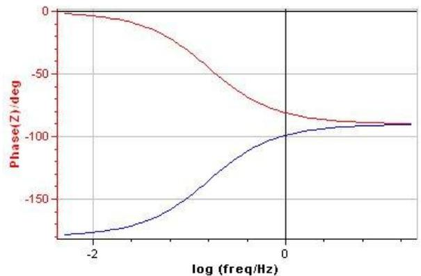
**Figure 9: Comparison of the impedance phase for  $R > 0$  (red) and  $R < 0$  (blue).**
