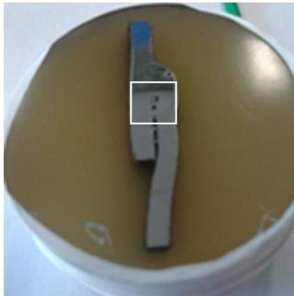
**Figure 4:** Picture of the welded steel used as a sample. The width of the welded part is 6.4 mm. The analysed area is outlined by the white square.
